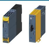
Hybrid technology provides reduced size, lower heat losses and longer service life in motor starter applications by combining relay contacts, power semiconductors and a solid-state overload relay.
